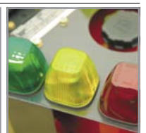
Overload warning lamps + auto stop + alarm
